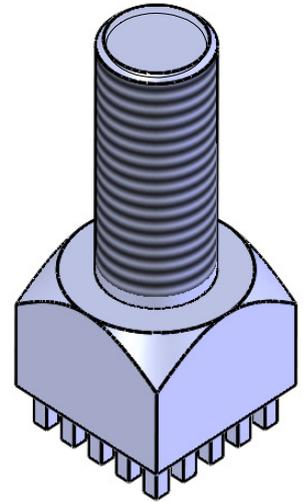
max. allowable torque for M8: 9Nm
