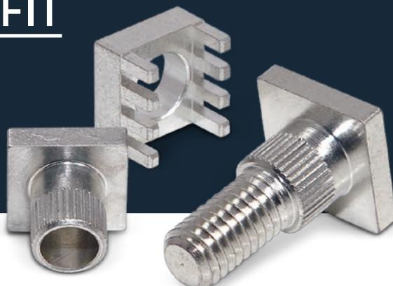
**PowerTwo Press-fit** Powerelements are two-piece high current contacts and a solution patented by Würth Elektronik ICS for the screw technology on PCBs. They enable a permanent and reliable connection or mounting on the PCB without adding stress. Depending on the pin arrangement and the corresponding layout, currents of up to 500 amperes are possible. The assembly method allows individual adjustments regarding dimensions.
