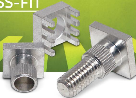
**LF PowerTwo Press-fit** Powerelements are two-piece lead-free high current contacts and a solution patented by Würth Elektronik ICS for the screw technology on PCBs. They enable a permanent and reliable connection or mounting on the PCB without adding stress. Depending on the pin arrangement and the corresponding layout, currents of up to 500 amperes are possible.
